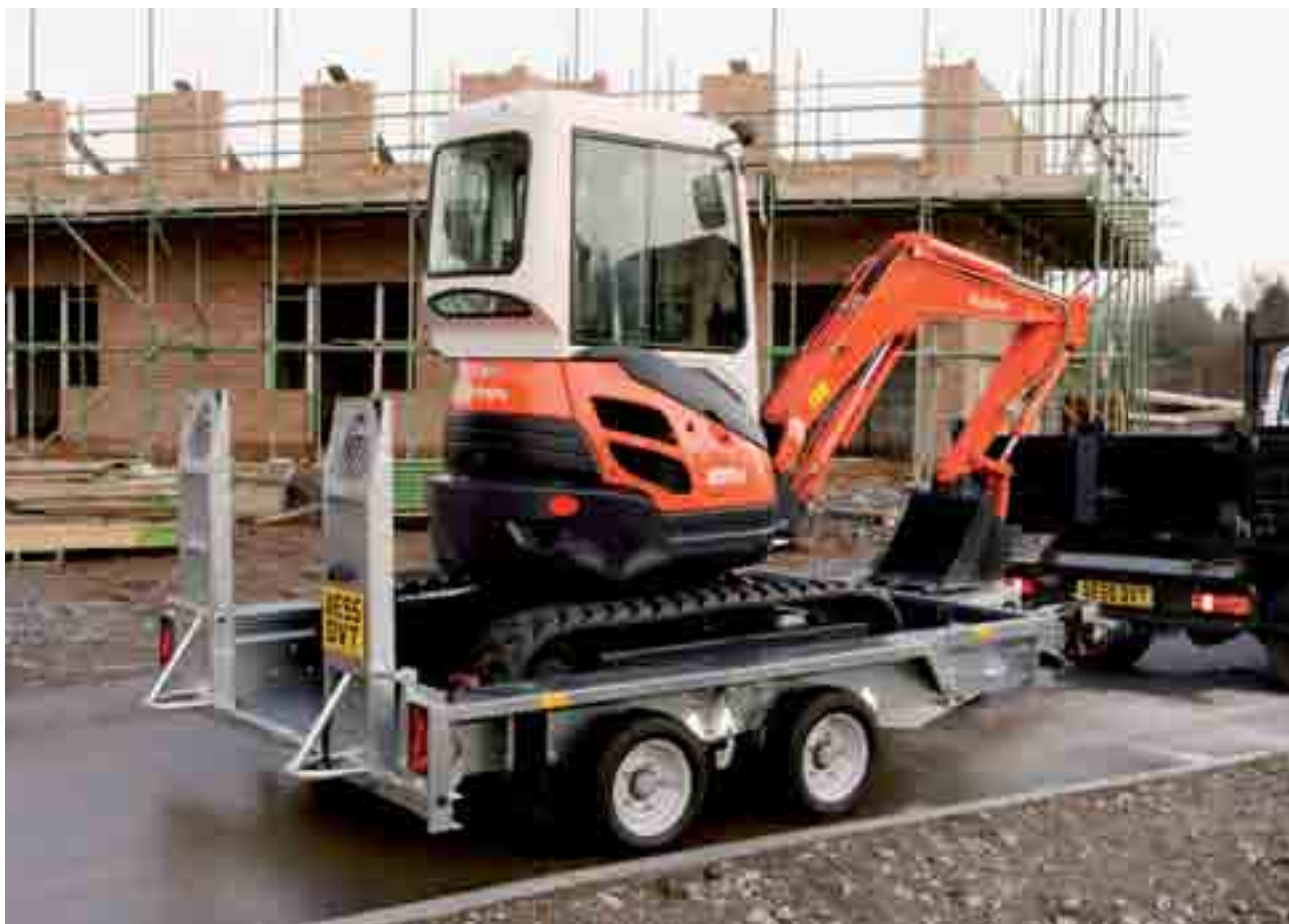
GX106 with skids and integrated rear supports
