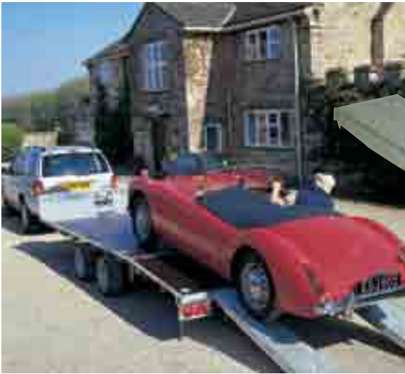
LM167/B with optional headboard, skids, electric winch, prop stands and lashing rings.
